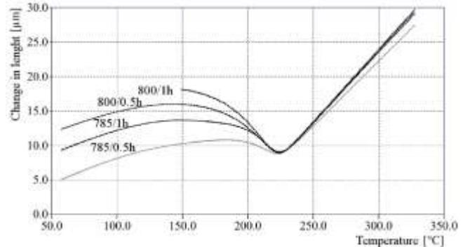
**Fig. 3** The effect of the temperature and the time of annealing in the intercritical range on the increase in the sample length during the martensitic transformation
