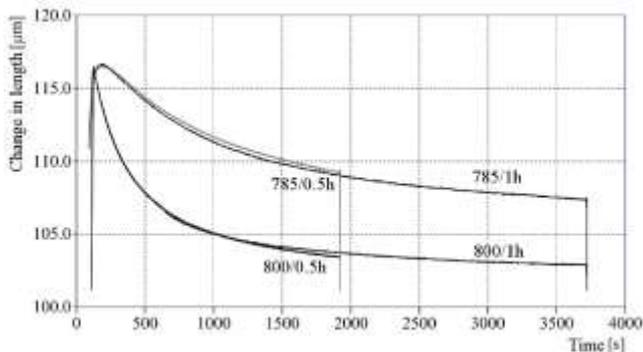
**Fig. 2** A change in the length of a dilatometric sample of 38CrAlMo6-10 steel during the intercritical annealing
