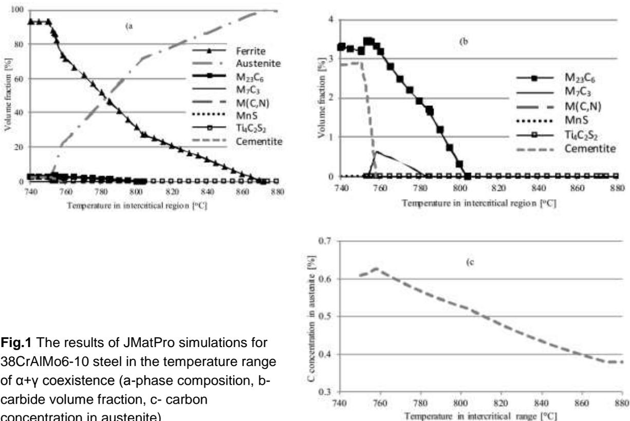
**Fig.1** The results of JMatPro simulations for 38CrAlMo6-10 steel in the temperature range of  $\alpha+\gamma$  coexistence (a-phase composition, b-carbide volume fraction, c- carbon concentration in austenite)
